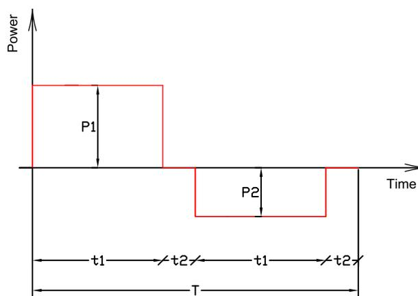
Fig. 2. Reference lift profile of a bridge crane.
