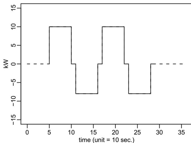
Fig. 3. Power curve with two cycles ( $m = 2$ ), shift 5 and  $T = 12$  during interval  $[tL, (t + 1)L)$ , corresponding to  $L = 3T = 36$ . The two cycles are drawn in solid line.
