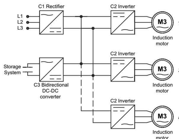
Fig. 1. Electric scheme of multiple bridge cranes supplied by a single main supply and a centralized storage system.
