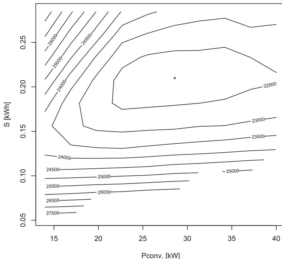
**Fig. 5.** Monte Carlo estimate of the expected value of the life-cycle cost, (5), with 5 drives and search region given by  $S \in (0.053, 0.284)$  kWh and  $P_{\text{conv.}} \in (14, \min\{360S, 40\})$  kW, with  $P_R = 50$  kW. The asterisk marks the point from the searching grid with minimal cost.
