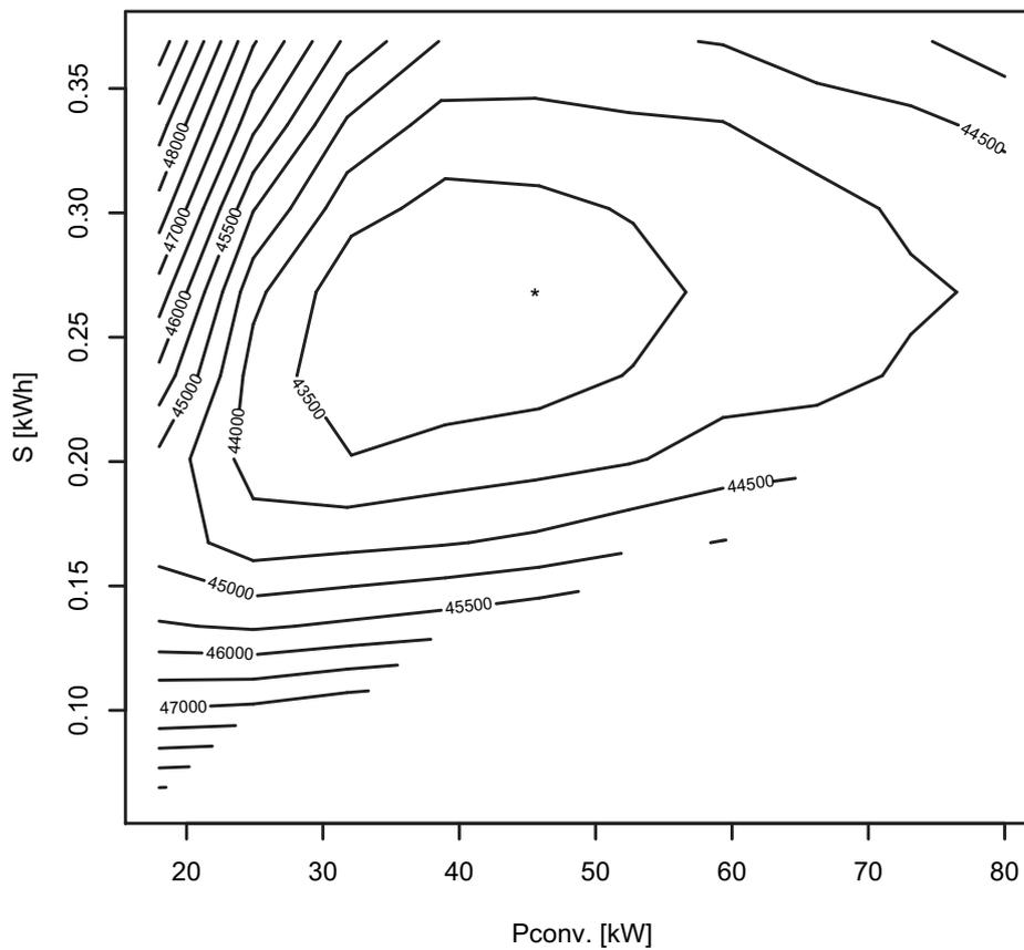
Fig. 4. Monte Carlo estimate of the expected value of the life-cycle cost, (5), with 10 drives and search region given by  $S \in (0.067, 0.369)$  kWh and  $P_{conv} \in (18, \min\{360S, 80\})$  kW, with  $P_R = 100$  kW. The asterisk marks the point from the searching grid with minimal cost.
