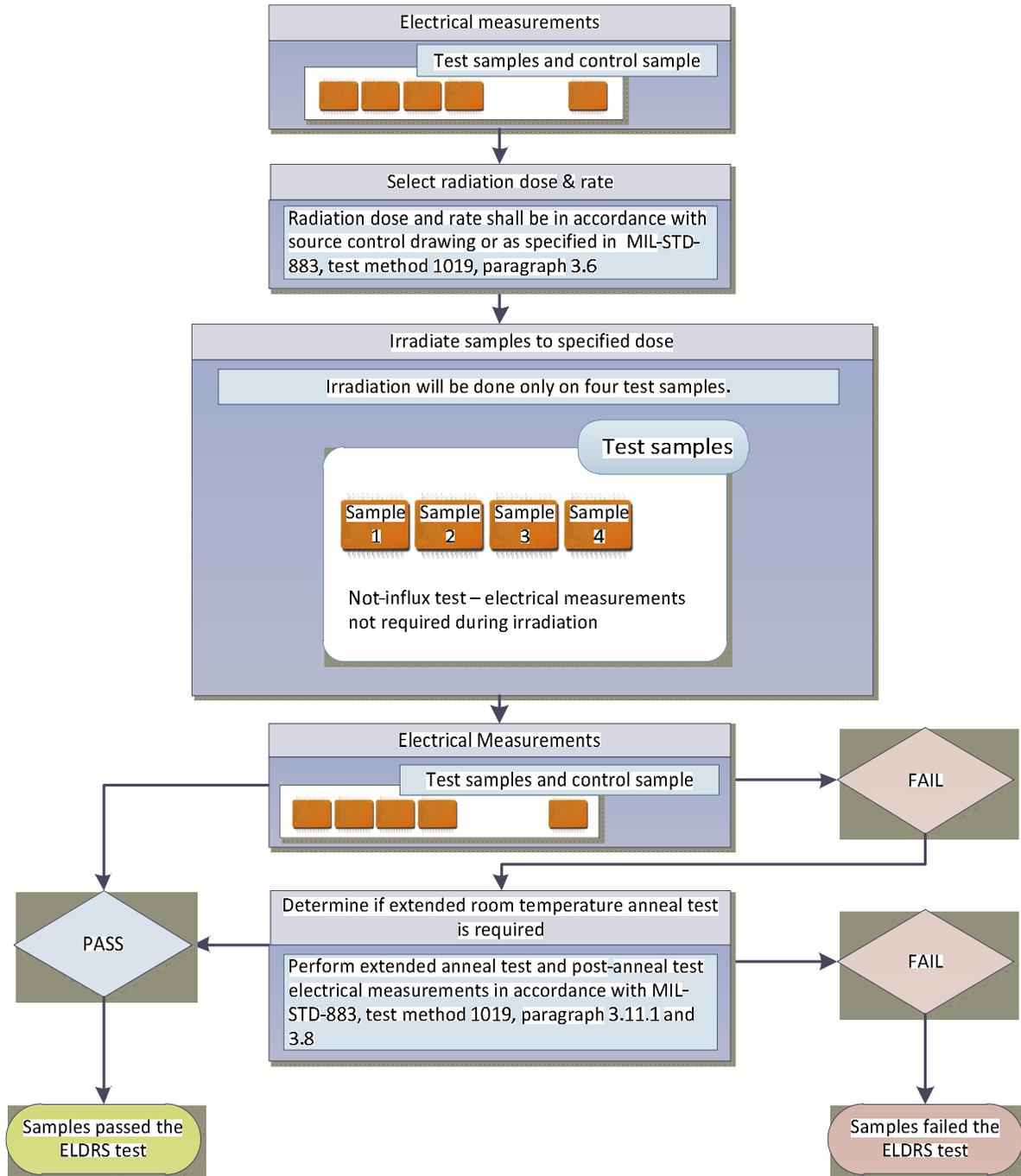
**Figure 8: ELDRS test flow diagram.** The figure illustrates sequence of the ELDRS test performance procedure. Adopted from (MIL-STD-883, 2010).
