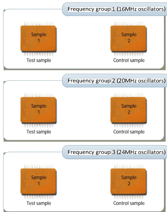
**Figure 9: Test sample size selection.** The figure illustrates samples used for radiation hardness testing. Samples are grouped into three different frequency groups. Each frequency group contains one test sample (used for irradiation) and one control sample (never being exposed to radiation).
