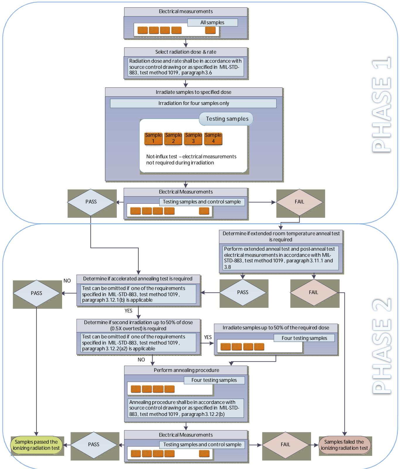
**Figure 7: Neutron and total ionizing dose test flow diagram.** The figure illustrates sequence of the ionizing dose test radiation. Adopted from (MIL-STD-883, 2010).
