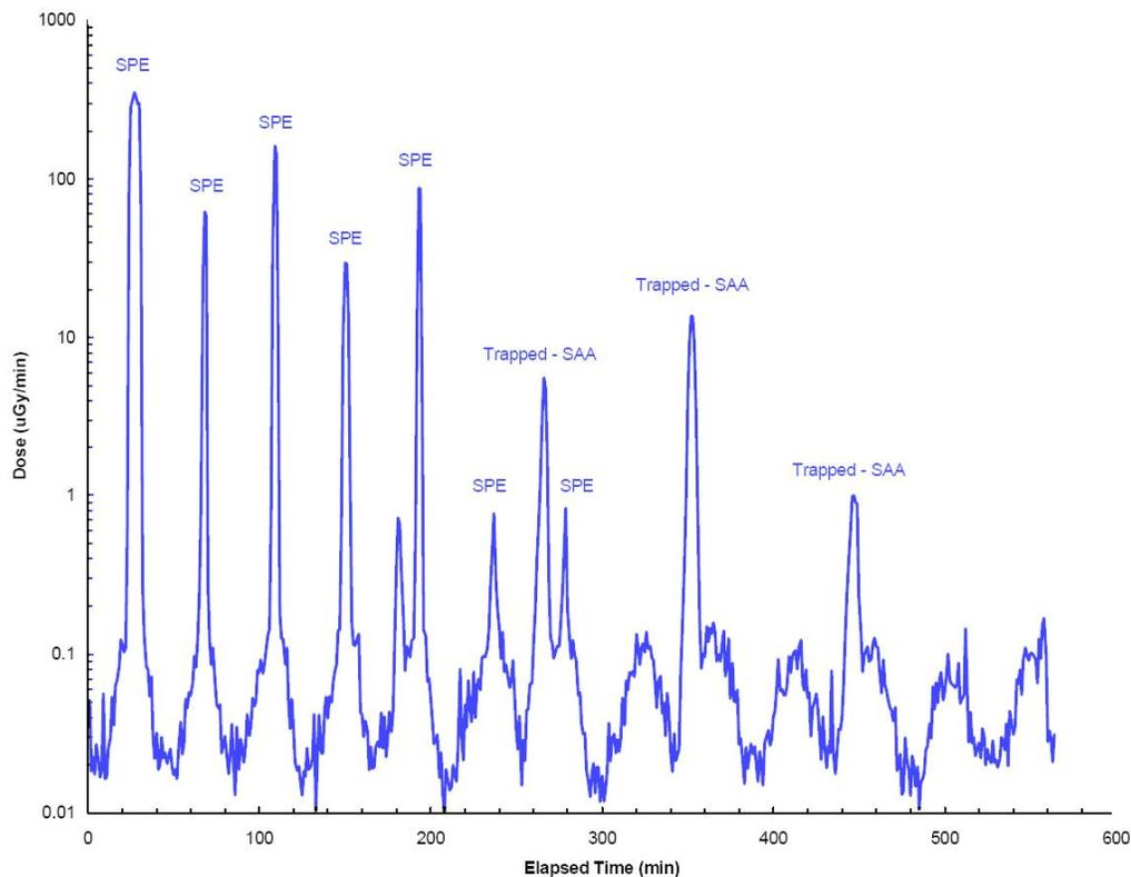
**Figure 2: Radiation measurements on ISS.** This graph shows radiation dose rate measurement versus time. Measurements were made on November 9, 2000. In addition to Solar Proton Events (SPE), graph indicates radiation measurements of trapped radiation from South Atlantic Anomaly (SAA). Adopted from (Shelfer, 2002).
