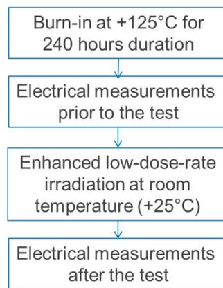
**Figure 5: The ELDRS test flow.** The test procedure for ELDRS requires irradiation dose rate less or equal to 10 mrad(SiO<sub>2</sub>)/s and burn-in prior to the radiation test. Electrical measurements are required before and after the irradiation process, as well (MIL-STD-883, 2010).
