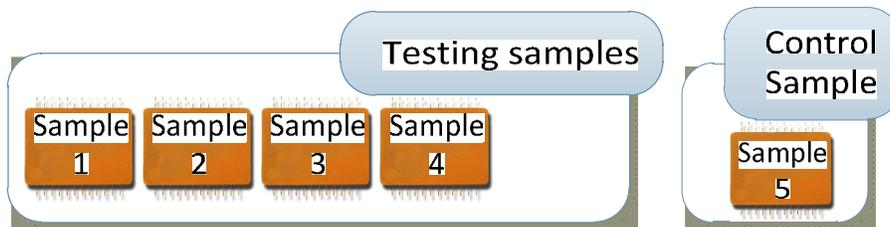
**Figure 6: Neutron and total ionizing dose test sample selection.** The figure illustrates two groups of test samples. First group is consists of testing samples and second group consists of control samples. Samples from both groups are electrically tested prior and after the irradiation process. However, the control sample is not irradiated and used to measure shift in electrical parameters of irradiated samples.
